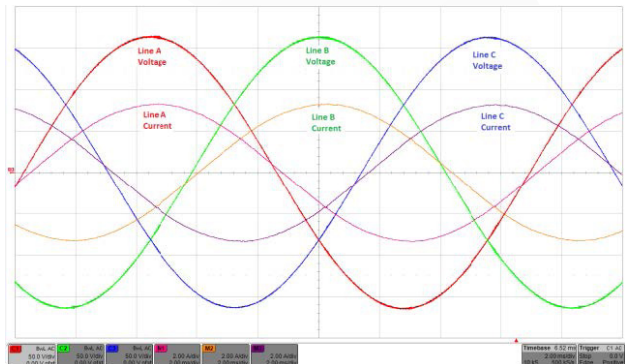
Figure 6. 60Hz, Full Load, 2 msec/div Line Voltage: 50 V/div Line Current 2 A/div
